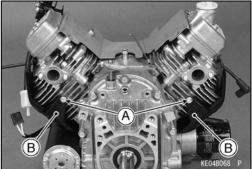
• Unscrew the rocker cover mounting bolts [A], and remove the cover [B] and gasket.
